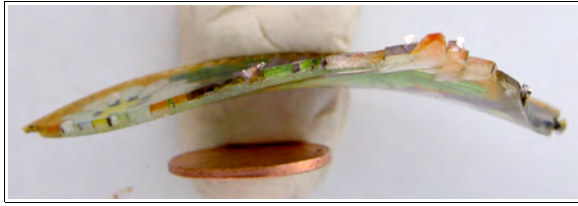
A piece of broken antique shōtai showing the thickness of the enamel compared to a penny
